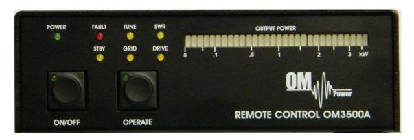
ON / OFF - Standard ON / OFF switch. On state is indicated by green LED on the switch
